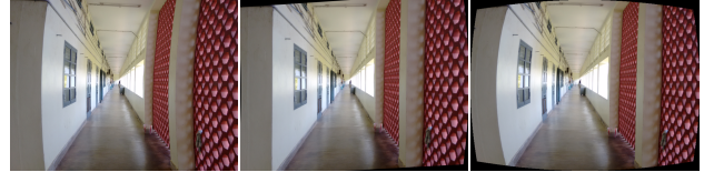
Figure 1. (a) Image curved due to RS effect, (b) rectified image in which curves are corrected to lines respecting the orthogonality of vertical and horizontal edges using the proposed method, and (c) rectified image using the lens correction method [35]
